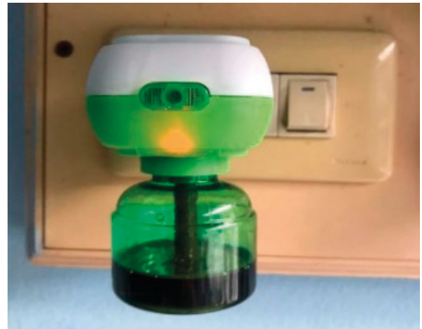
Figure 1 An electric mosquito-repellent machine contained herbal mosquito repellent essential oil
