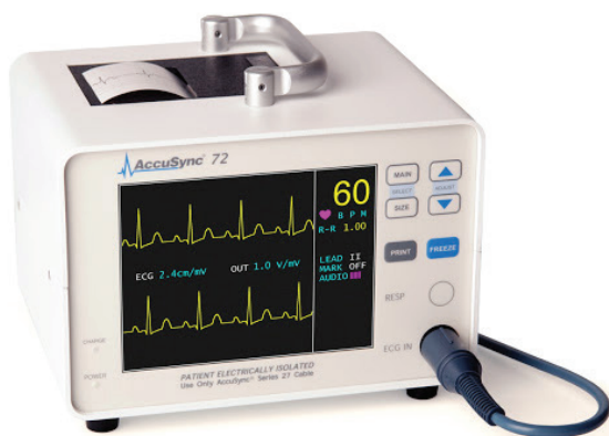
รูปที่ 6 The Accu-sync ECG-gating device (model 72; Milford, Connecticut) connected to a 5-lead ECG to allow IRE pulses to be synchronized with the refractory period of the heart to avoid arrhythmias
