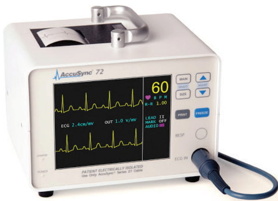
รูปที่ 6 The Accu-sync ECG-gating device (model 72; Milford, Connecticut) connected to a 5-lead ECG to allow IRE pulses to be synchronized with the refractory period of the heart to avoid arrhythmias
