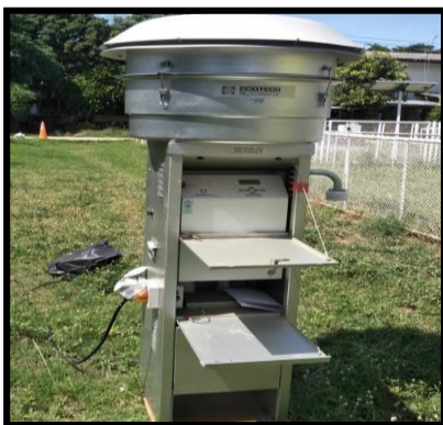
(ก) PM 2.5 High Volume Air Sampler
