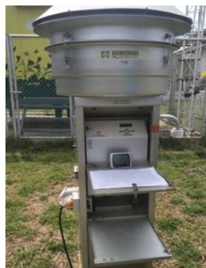
(ข) PM_{2.5} High Volume Air Sampler
