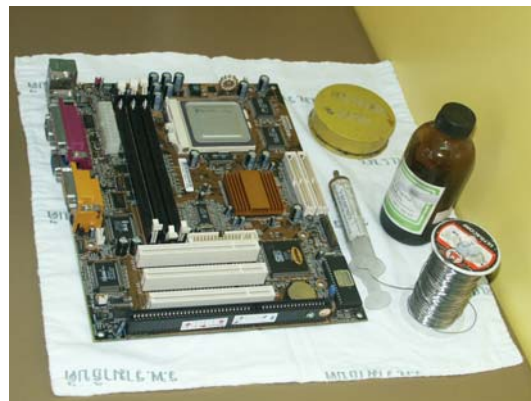
Figure 3 Computer main circuit board; solder paste in syringe and yellow case, bottle of liquid flux and flux cored solder wire
