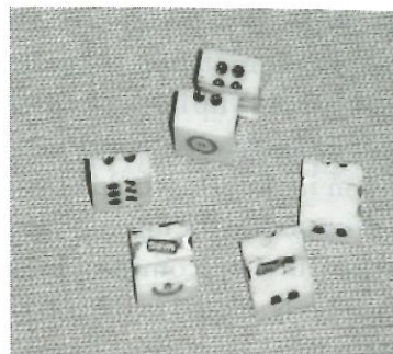
Figure 5 Cross-section of three dice bought legally from the market demonstrated implantation of magnets.
