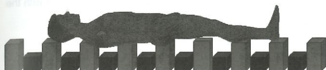
Figure 3 When movable parts move to their highest position, it could hold the entire patient's weight.
