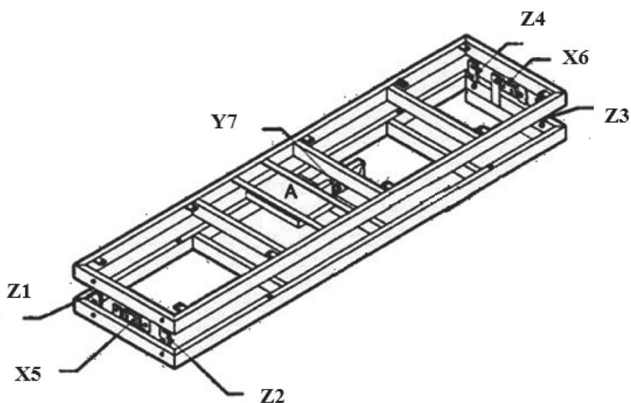
**Figure 1:** Positions of load cells mounted to the couch frame Z1 to Z4, X5 to X6 and Y7 represent the location of the four load cells in the vertical, two load cells in medial-lateral and one load cells in caudad-cephalad directions, respectively. A represents the amplifier.
