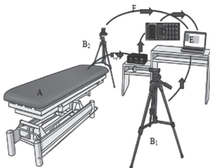
**Figure 2:** Functional processes of the data obtained from the instrumented couch and two cameras flow to the computer.
