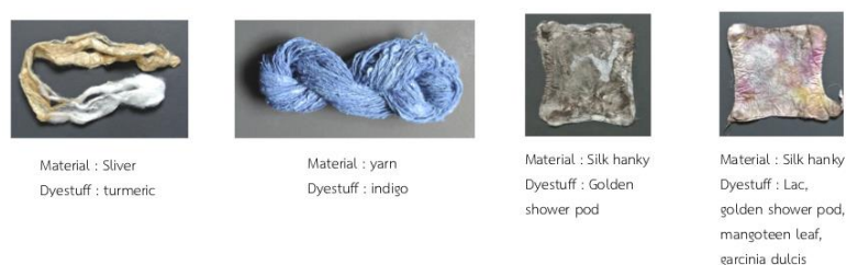
Figure 9. The sample of dyeing outcomes from different material and dyestuffs.
