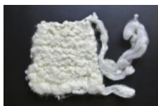
Figure 11 : Knitted fabric from silk hankies sliver produce by hand knitting needle no.8.
