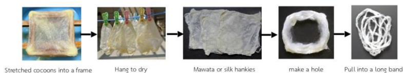
Figure 5. The process of turning cocoons into mawata or silk hankies and roving.
