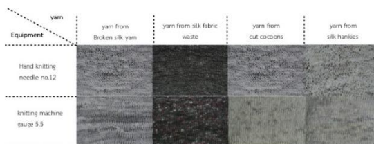
Figure 12 : Knitted fabric produced from Thai silk waste yarn by hand needle and knitting machine.
