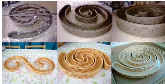
Figure 14 : firing at 1,200 Celsius.
