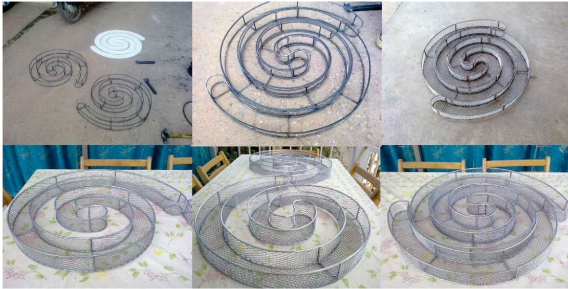
Figure 16 : used to construct with 6 millimeters dense steel rod.
