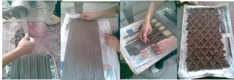
Figure 12 : Then, it is woven as Kid motif and undergone biscuit and bake firing at 1,200 Celsius.
