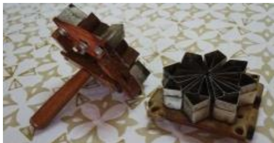
Figure 16: Modular batik block
