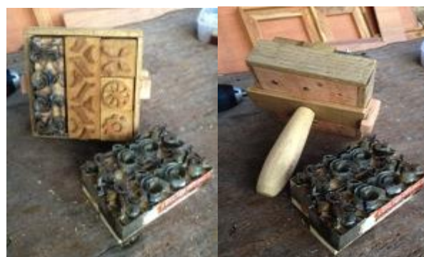
Figure 6: Example of Modular batik block type 1
