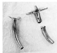
Figure 2 Fractured tracheostomy tube removed from the patient
