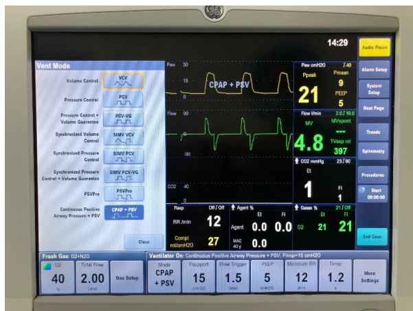
Figure 2 The Avance CS2 in CPAP + PSV mode, CPAP=continuous positive airway pressure, PSV=pressure support ventilation
