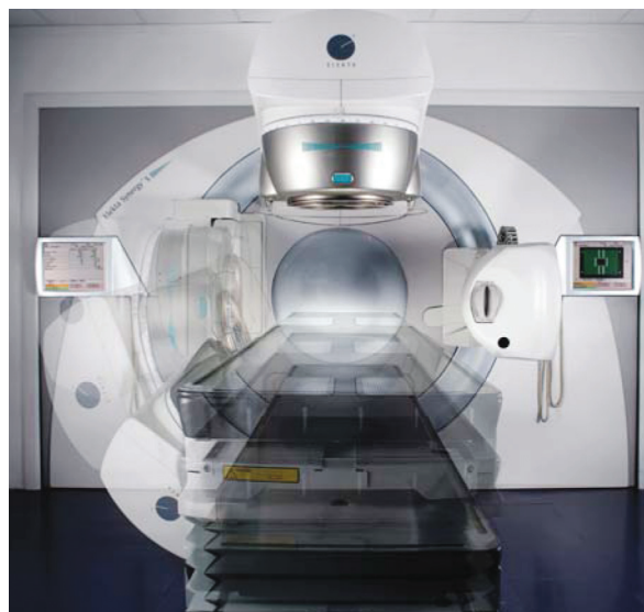
Figure 7: The Elekta Synergy ® combines VMAT&IMRT and image guided radiation therapy (IGRT), XVI ®
