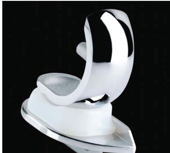
Figure 3: The tibial components are made from cobalt chromium molybdenum alloy. Six sizes are available for both the left and right side, for maximum coverage on tibial bone cut and to avoid anteriomedial overhang, which sometimes caused postoperative pain in the Phase 2 design.
