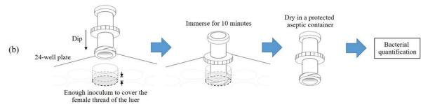
Figure 2: Inoculation with (a) the Inocap method; and (b) the traditional dip method.
