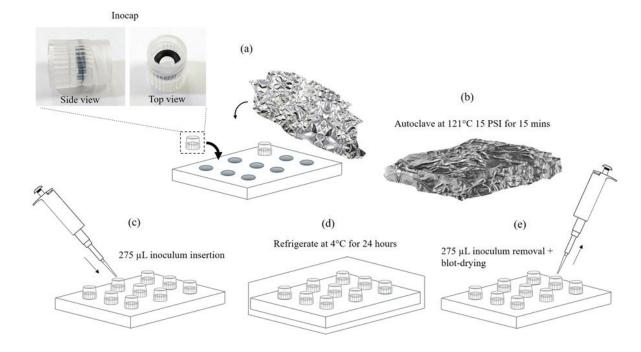
**Figure 1:** Inocap preparation process (a) picture of an Inocap and their placements on an autoclavable tray wrapped by aluminium foil; (b) caps sterilization; (c) addition of bacterial stock; (d) refrigeration in a sterile box; and (e) inoculum removal.
