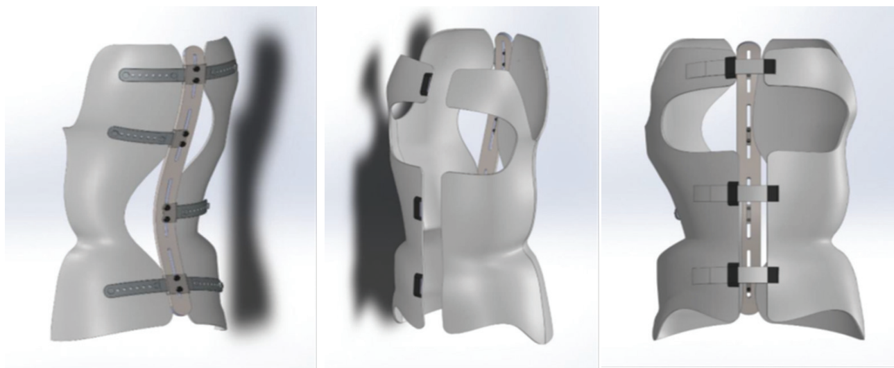
Figure 2: Assembling the designed brace in Solidworks software
