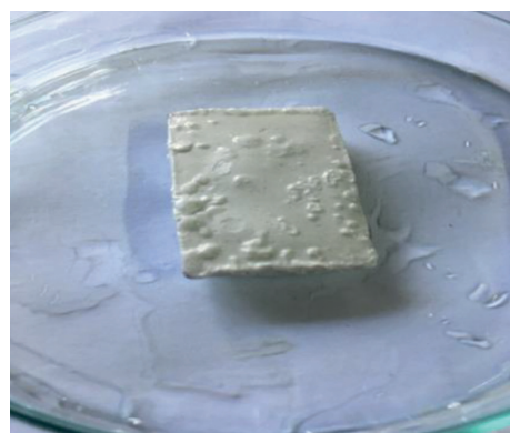
Figure 8 Artificial skull parts after immersion testing
