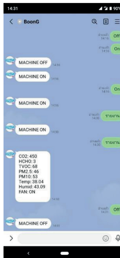
Figure 3 LINE messenger was used to send direct messages for air cleaner control.
