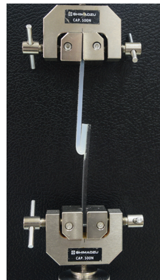
Figure 4 Specimens position in Universal testing machine during peel bond test.
