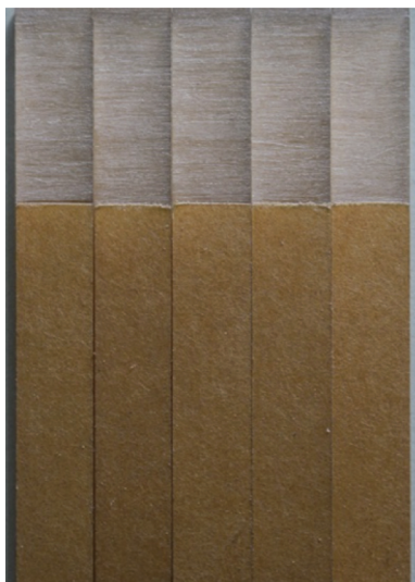
Figure 3 Surface preparation of plexiglas acrylic strips
