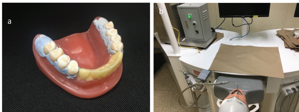
Figure 2 (a) Mandibular dental model with premolar tooth samples placed at the posterior regions; (b) Phantom head attached with water pump
