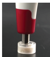
Figure 3 Specimen was measured using VITA Easyshade V at 4 points perpendicularly via measuring jig.
