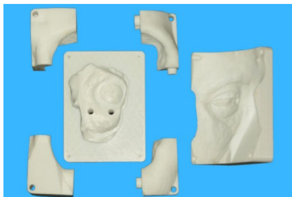
Figure 5. 3D Printed Indexed 6-Piece Negative Mold for Fabricating Silicone Orbital Prosthesis
