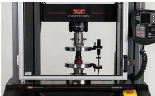
Fig 3. universal testing machine/shearing/tensile/compression 5960 series)
