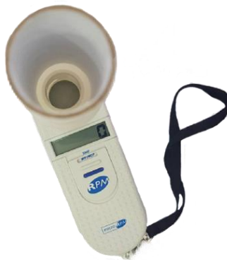
Figure 2 MIP measurement device with single-use cylindrical paper mouthpiece
