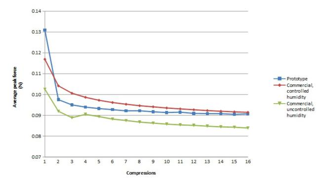
Fig 5. Average peak forces of commercial monofilaments in both indoor humidity condition and controlled condition with fixed humidity at 45% and prototype monofilaments in controlled condition with fixed humidity at 45% after 16 consecutive compressions.
