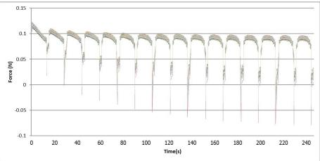
Fig 3. Forces of 16 consecutive loading, unloading, and resting pattern of commercial monofilaments put in controlled condition with fixed humidity at 45%.
