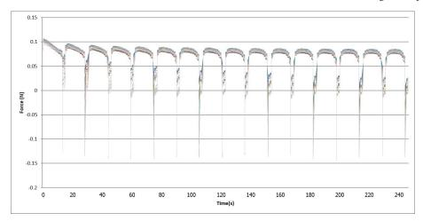
**Fig 2.** Forces of 16 consecutive loading, unloading, and resting pattern of commercial monofilaments put in indoor humidity condition.
