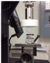
**Fig 1.** Commercial monofilament (left) and prototype monofilament (right) on a universal testing machine for compression test to simulate sensation testing on the patient's foot.
