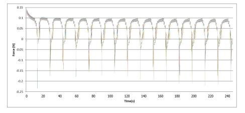
Fig 4. Forces of 16 consecutive loading, unloading, and resting pattern of prototype monofilaments put in controlled condition with fixed humidity at 45%.
