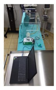
**Fig 5.** The set up for testing PM leakage from the opening with glove attached. The burning incense stick can be seen in the endoscopic aerosol box and the two PM sensors are placed inside the aerosol box and the sealed compartment attached to the endoscope-glove opening respectively.
