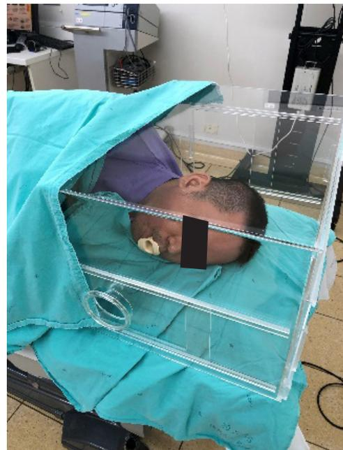
**Fig 2.** The transparent endoscopic aerosol box, showing the opening for the scope (An endoscopy unit staff is modeling as the patient).
