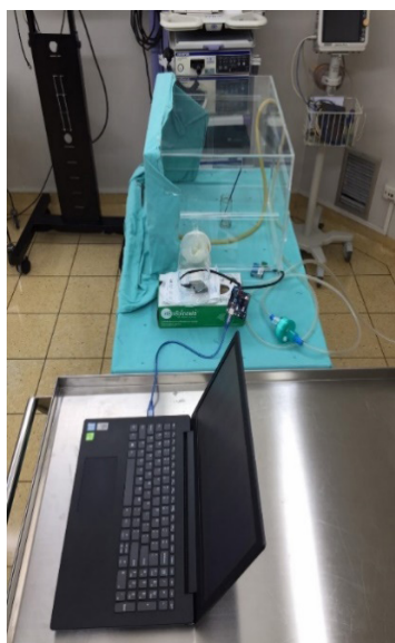
Fig 5. The set up for testing PM leakage from the opening with glove attached. The burning incense stick can be seen in the endoscopic aerosol box and the two PM sensors are placed inside the aerosol box and the sealed compartment attached to the endoscope-glove opening respectively.
