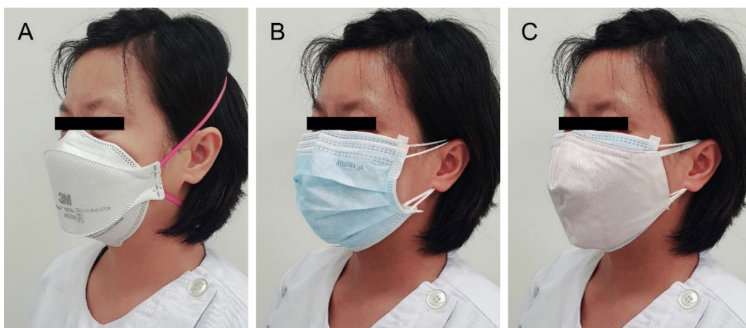
Fig 1. Three mask wearing scenarios tested: (A) NIOSH-approved N95 mask without a valve, specifically the 3M™ 1860S, (B) medical surgical mask, double-layered, and (C) three-tiered medical surgical mask covered by a cloth face mask.
