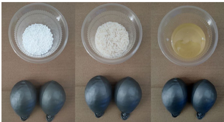
Fig 3. The pads were created by filling small latex bags with various materials: polystyrene ball bullet foam (left), uncooked jasmine rice (middle), and sugar cane syrup (right). The images show the materials before filling the pads (top row) and the completed pads (bottom row).
