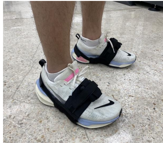
Figure 2 Placement of the F-sensor on the Runner's Shoes.
