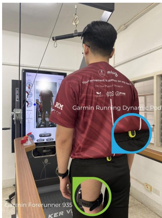
Figure 1 The fitness watch (Garmin forerunner 935) was worn on the habitual hand, and the accelerometer (Garmin Running Dynamics Pod) was attached to the pant.
