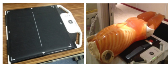
Figure 1. (A) Digital flat panel detector with grid manufactured by GE. (B) The whole-body phantom KYOTO KAGAKU model-60.
