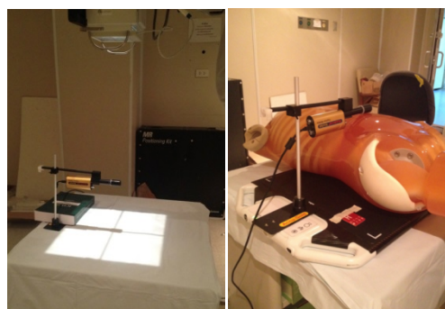
Figure 2. (A) Incident air kerma, K_i , measurement and (B) ESAK measurement for 21 cm thickness of abdomen in phantom.
