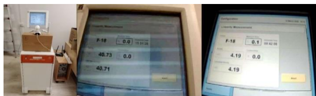
Figure 4 (Left) Close circuit camera was used to record screen display. (Middle) Screen display at beginning (Right) Screen display after 6 hours.
