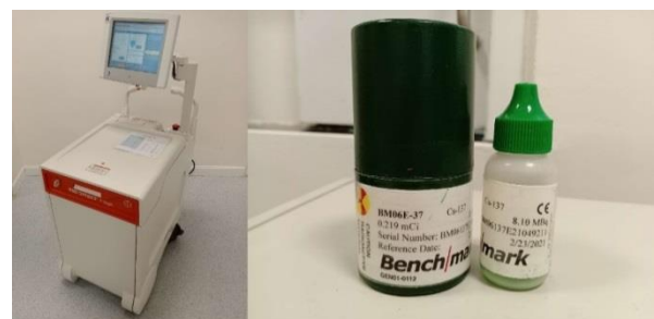
Figure 3. MedRad Intego PET infusion system and ^{137}\text{Cs} reference source used in quality control.
