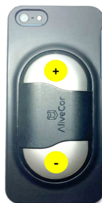
Figure 1 An iPhone ECG heart monitor (Alivecor veterinary heart monitor) cased on iPhone 5s (iOS 10.3.4), the negative electrode is located lower of the case and the positive electrode is located upper of the case.
